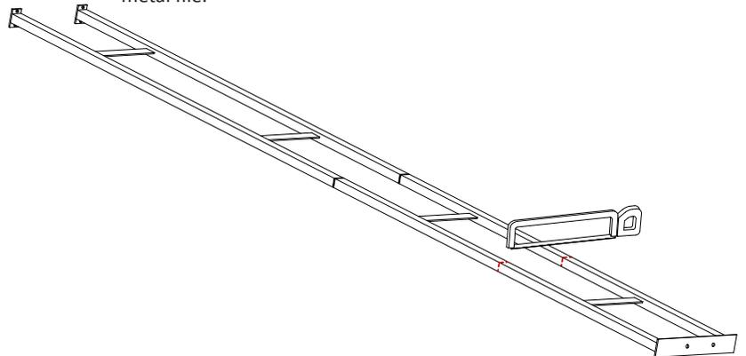
5. **Complete the installation** - Install the second set of FCF-HIDDEN following the procedure in step 3 and refer to the Floor to Ceiling Frame (FCF) installation instructions to complete the remaining installation steps, ensuring that screws are securely fastened into both mounting holes in each FCF-HIDDEN bracket.
