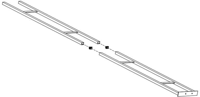
3. **Insert the FCF-HB pieces** - Slide the FCF-HIDDEN pieces into the open ends of the Floor to Ceiling Frame, with the mounting holes positioned toward the front and back of the Frame as shown below. For maximum rigidity when installed, it is recommended that a self drilling screw be inserted through the side wall of the frame and into the "U" channel of each bracket.
