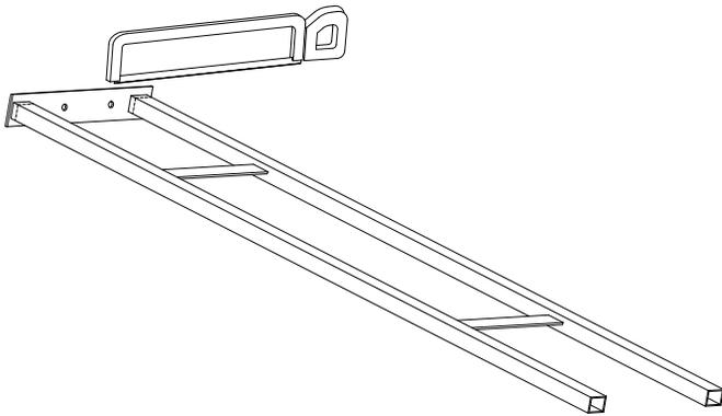
2. **Assemble the frame** - Locate the plastic couplers that came with the FCF-HD and insert them into the open end of one section of FCF-HD. Taking care to appropriately protect the frame and your work surface / floor from damage, slide the two sections of FCF-HD frame together, so that the couplers are fully seated in both sections of the FCF-HD.
