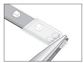
Use a small section of shrink tubing to seal cut ends. While the tube is still warm, lightly pinch the end with pliers to seal. Glue should ooze from the end.
