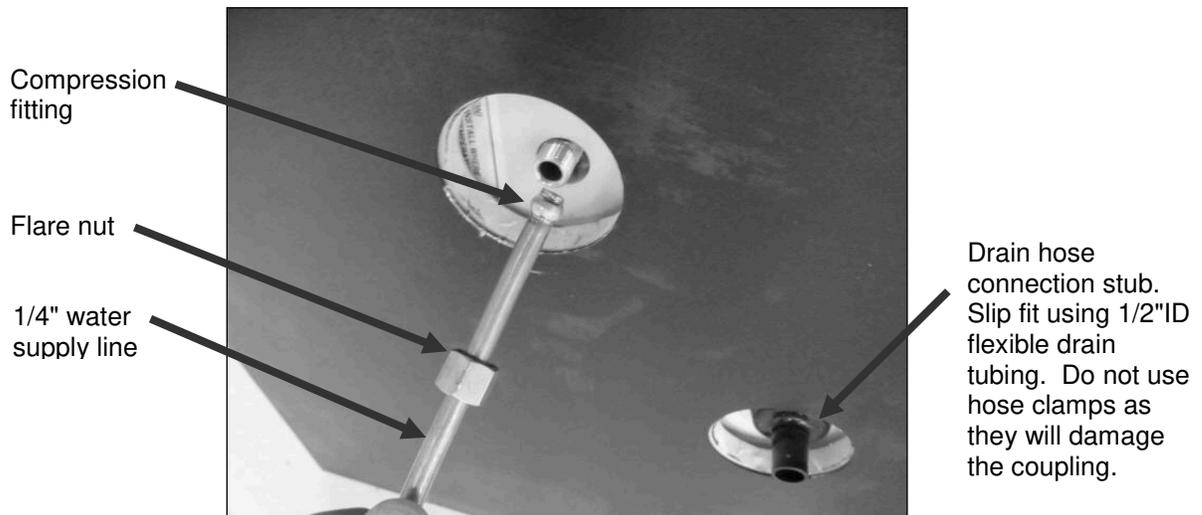
Use two wrenches when tightening water line to avoid damage to the internal water solenoid valve.
